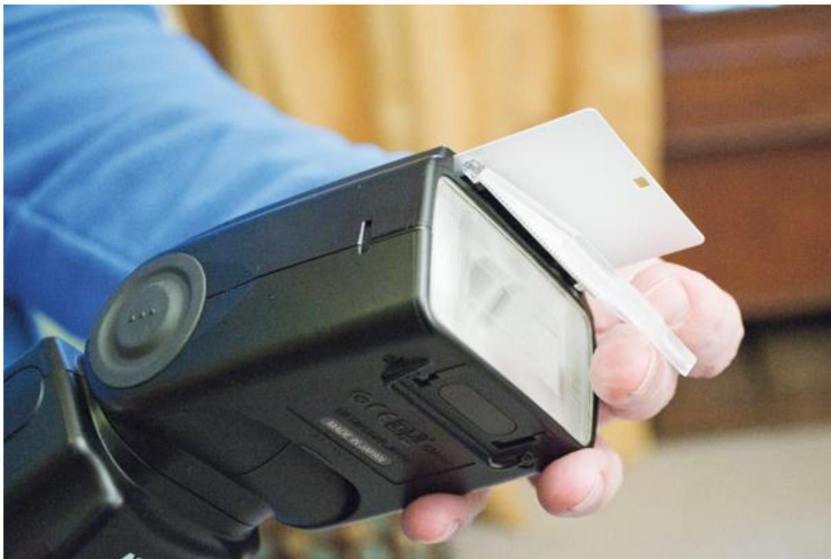
Better flashguns have a white bounce card built into the flash head to reflect some light directly onto the subject when the unit is tilted up into a bounce position.
