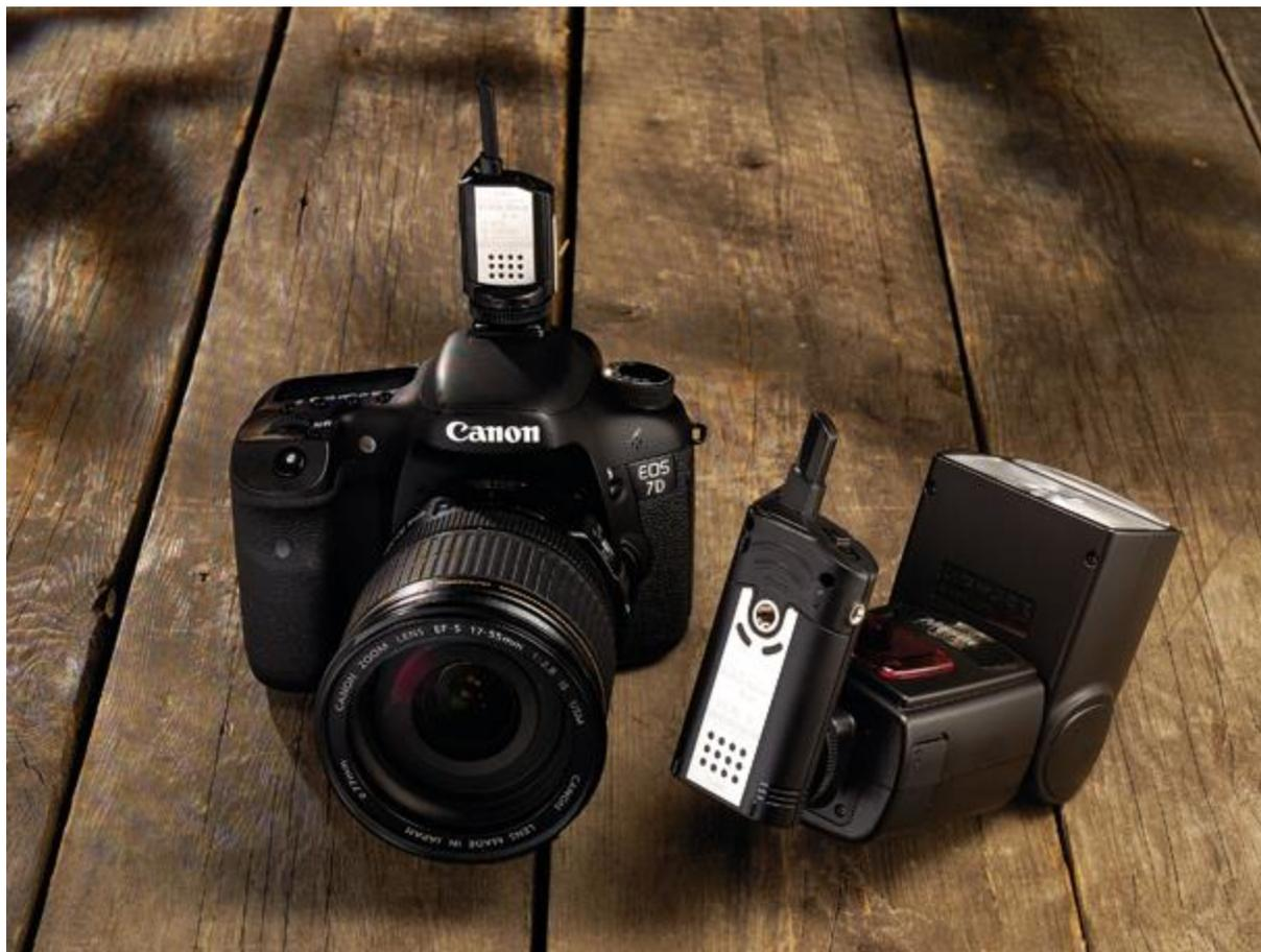
Using two or more flashguns will extend your lighting options considerably. To avoid nasty multiple flash exposure calculations and cumbersome cord connections, the simplest, most effective way to connect several flashguns is via a wireless TTL multi-flash system.
