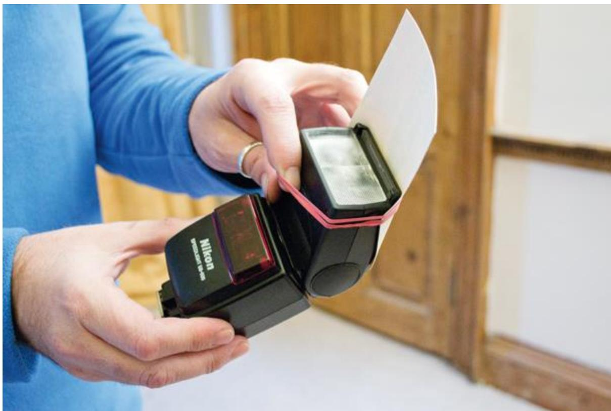
If your flashgun doesn't feature a bounce card or dual flashtube, try using a rubber band to secure a piece of white card around the back of the flash head to reflect some light forward.
